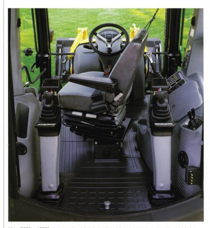
With a ROPS and FOPS structure and a modern design, the cab features a top class automotive style. Its increased internal volume and wide round glass surface offer great comfort to the operator. The De-Luxe suspension seat is standard.
