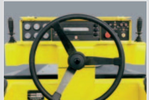
Dual levers control travel direction, speed, manual vibration on/off and MSPI input from either seating position.
