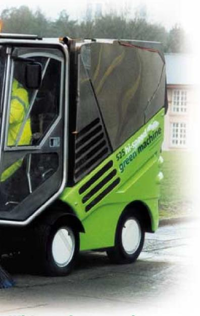
Ideal for sidewalks. The joystick-controlled brushes scour debris from in and around tight areas.
