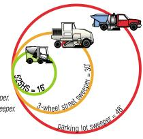
The 525HS has double the maneuverability of a typical three-wheeled street sweeper.
