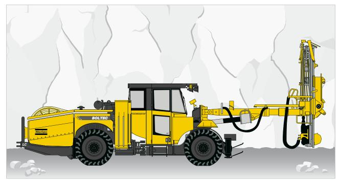
A diesel hydraulic, fully mechanized rock bolting rig with RCS based control system for high productivity and precision. For bolt lengths 1.5–6 m and effective in roof heights up to 12 m.
