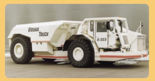
**Kiruna Truck K 503** for mining and tunnelling. The K 503 is an articulated, heavy duty, low profiled truck for underground haulage. The trucks are designed to allow biggest possible volume with smallest outer dimensions. The trucks are equipped with wet disc brakes and for excellent driver's comfort, front axle is suspended with shock absorbers and rubber elements.
