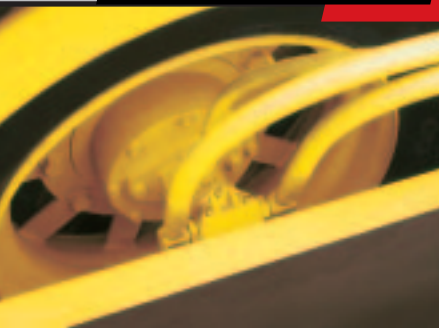
Radial pneumatic isolators ensure vibratory energy is transmitted to the work, not the machine
