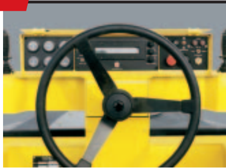
Two levers control travel direction, speed, manual vibration on/off and MSPI input
