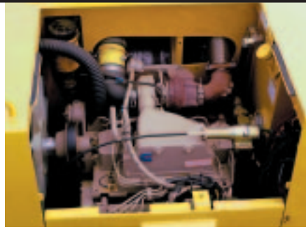
The engine is placed low in the frame for ease of service and operator visibility
