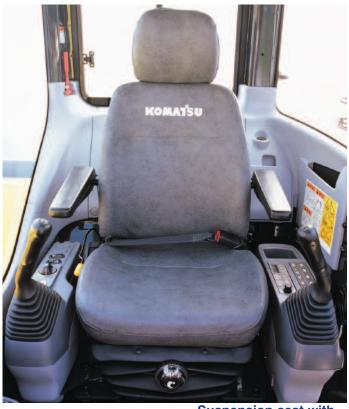
Suspension seat with retractable seat belt
