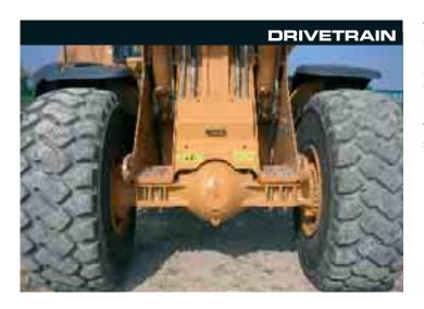
The 921E uses a torque sensing autoshift transmission, offering manual or fully automatic control. Both axles incorporate limited slip differentials for maximum traction when digging and loading. Axles feature optional oil coolers with continuous flow and filtration. Disc brakes are oil cooled for maximum retardation and reduced heat build-up, prolonging brake component life and reducing operating costs.
