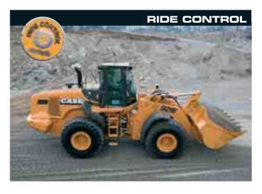
The ergonomically designed Case wheel loader can be specified with Ride Control, a system that allows the lift arms to float when the machine is moving. This reduces shock loadings on the operator and the machine, reducing fatigue and prolonging component life. Ride Control allows the operator to drive at higher speeds during load and carry operations, offering excellent load retention of material, for maximum productivity.
