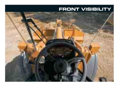
The 921E has an ergonomically designed cab that is far larger than on its predecessor. Pillarless top to bottom glazing to the front and both sides of the cab offers an excellent view of the bucket corners or attachment.
