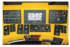
The new TEC° Plus electronic control system features CAN bus technology, which utilizes multiple control modules located throughout the machine for real-time performance data and advanced troubleshooting capabilities.
