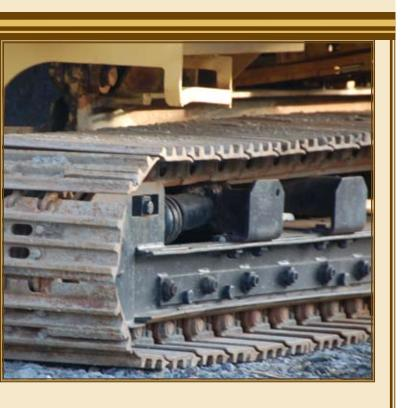
The track system of the T-800B provides the heavy-duty foundation necessary for the arge machine. For working in the dirtiest of conditions, the final track drive is completely enclosed. The track is spring-loaded to absorb shock load on the track system and to prevent the track chain from jumping the drive sprocket. Semi-cleated track pads 21" wide give you the flotation and traction you need.
