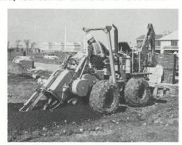
With the trencher attachment you get a torque adjustable slip clutch, a hydraulically controlled 'angle of attack' and an optional 20" end idler.
