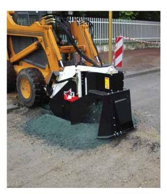
Particularly effective cutting thick layers of asphalt, concrete and rock, cuts clean without the damaging and uneconomic bordering caused by other equipments.
