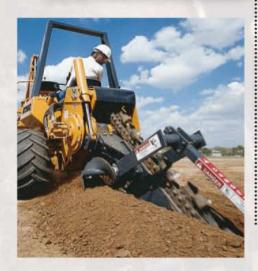
This optional attachment is available with a hydrostatic direct drive or planetary drive with either a standard sprocket or heavy-duty rock boom. Cupped or rock & frost teeth can be equipped on a standard or anti-backflex chain - crumber and restraint bars to match operating conditions.
