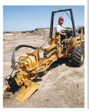
The P75 vibratory plow is designed as an integral part of the base tractor, yet removable for attachment versatility and greater utilization. Plow features, such as rubber iso-mounts insulate the operator from vibration. A hydraulic-swing plow frame with float position allows the plow to pivot back and forth a full 60° for maximum maneuverability in tight turns and to follow the path of least resistance in hard ground conditions.
